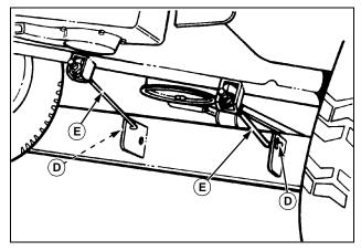
7. Remove spring locking pins and washers (D) from front draft rods (E) and remove draft arms from front axle brackets. Store draft arms with mower.
